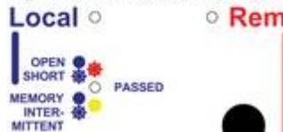
d) A short between two adjacent pins which have connections at both ends of the cable (Fig11).
